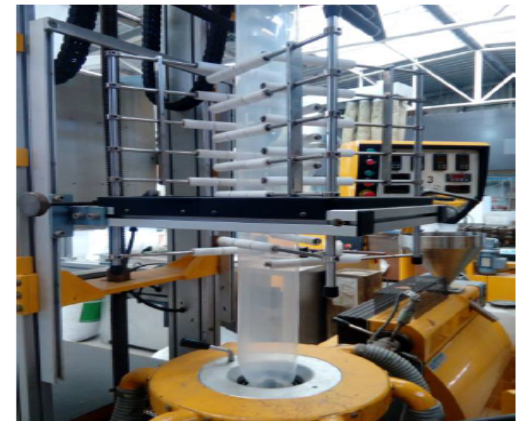
Figure 1. Co-extrusion of biodegradable bags
