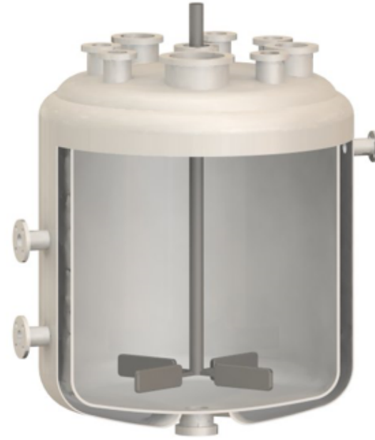
Pyrolysis reaction (400-500 °C) 50-100 mbar
