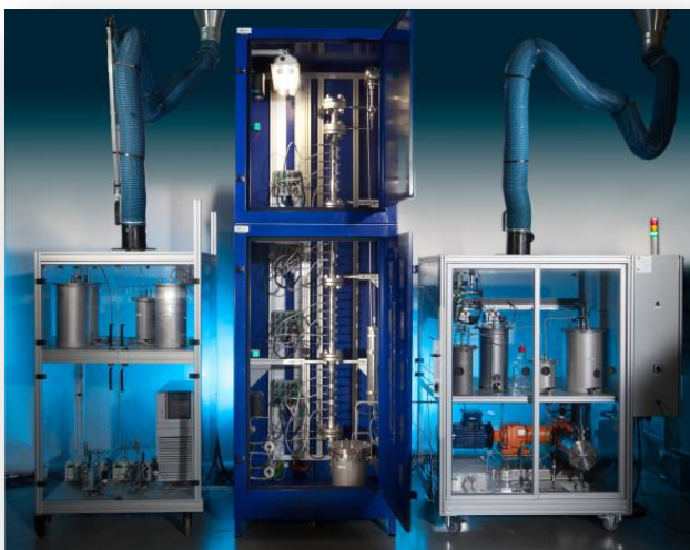
Biphasic reactor for conversion of waste into furans (kg/hr) 15
